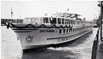
Britannia , 1,174 tons displacement, uses her bow-thrust device to manoeuvre out of a quay in tricky Rhine currents. She is 110 metres long for a breadth of only 11.6 metres overall, and 9.5 metres above the waterline for a draught of 1.41 metres. Her main machinery, aft, is four 425-hp marine diesels, coupled in pairs to two Voith-Schneider propellers.
